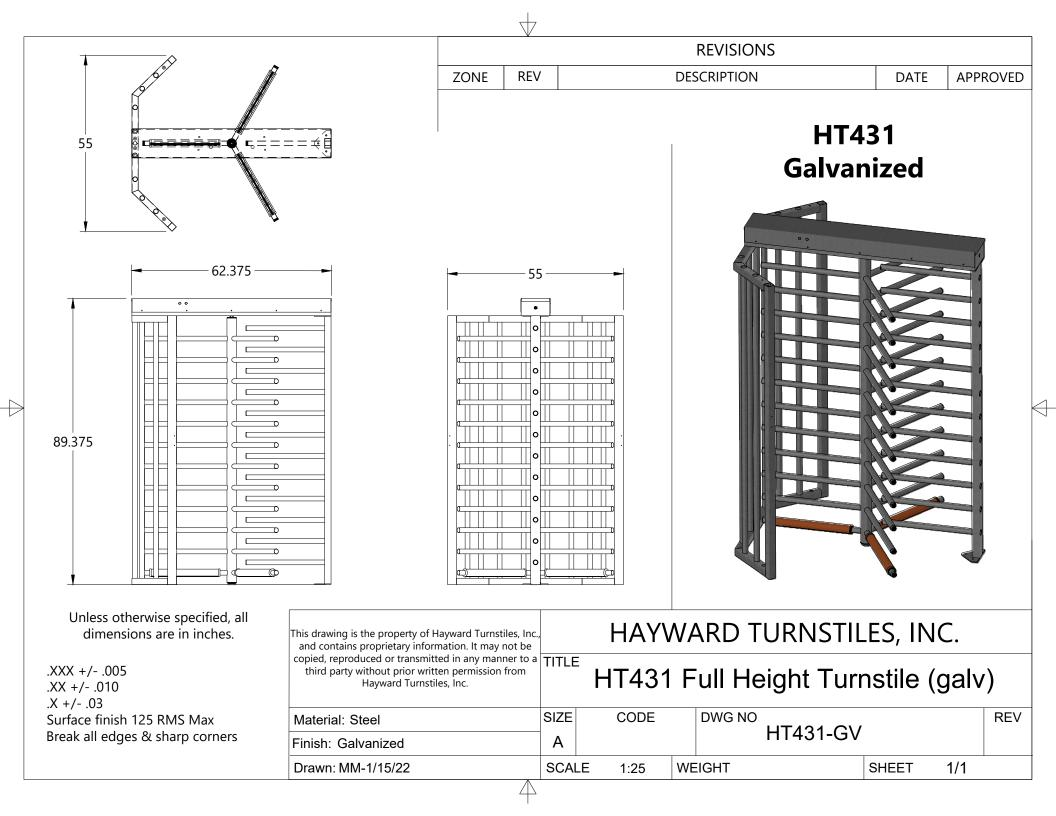
All measurements are referenced from the center of the rotating arm assembly.
